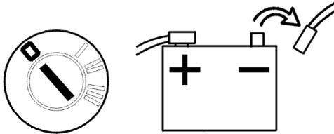
**Warning!** The SRS (supplemental restraint system) is active for a certain time after the power is cut. Therefore wait three minutes before starting work.
