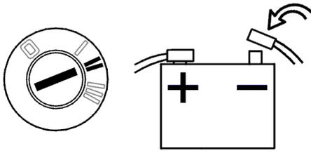
**position 2. No one must be in the car when the battery is connected. This is a safety precaution in case an airbag module activates when the power is connected.**
