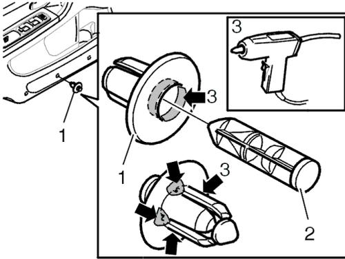
**Note! Certain inner door sides do not have a hole for a clip. These door panels must be modified. Take a correctly coloured door clip. Cut off the clip. Bond the clip to the door. Do not forget the centre section of the clip.**
