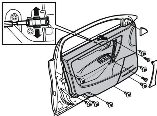
Remove the cover from the mirror by pulling it straight outwards. Detach the side piece handle at the bottom edge. Use a weatherstrip tool.
